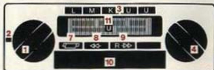
Radio with push buttons for band selection and tuning of preset stations and with built-in cassette player
