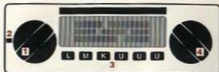
Radio with push buttons for band selection and tuning of preset stations
